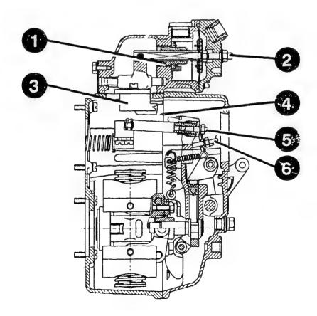
\* Lug cam with torque control
